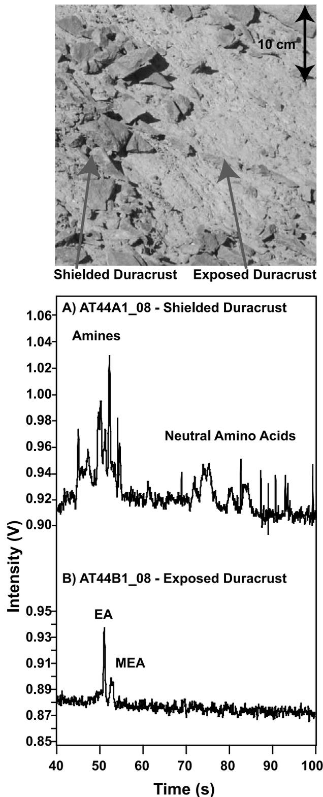
**Figure 2.** (top) Photograph of Site 44, showing the shielded and exposed duracrust areas. Samples were taken from the shielded duracrust and from the exposed duracrust at different depths at this site. (bottom) CE analyses of the surface extracts ( $<1$  cm) from this site analyzed in the field. The (a) shielded duracrust contained higher levels of neutral amino acids and amines, while the (b) exposed duracrust exhibited low levels of simple amines at the level of the solvent blank.
