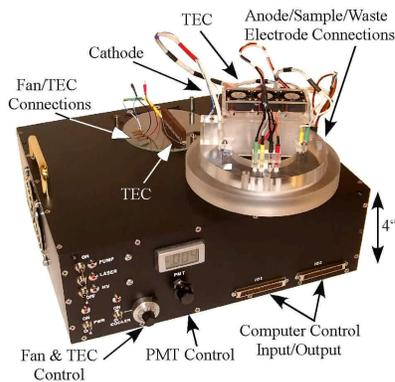
**Figure 2.** The Mars Organic Analyzer (MOA). The portable CE instrument, measuring 4" x 10" x 12", integrates all necessary pneumatic actuation, high voltage power supplies and confocal optics for laser excitation and fluorescence detection.
