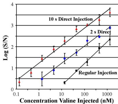
**Figure 3.** Limits of detection of the MOA system. The cross injection can detect down to 13 nM valine, the 2 second direct injection limits are 1.3 nM, and the 10 second direct injection limits are 130 pM.
