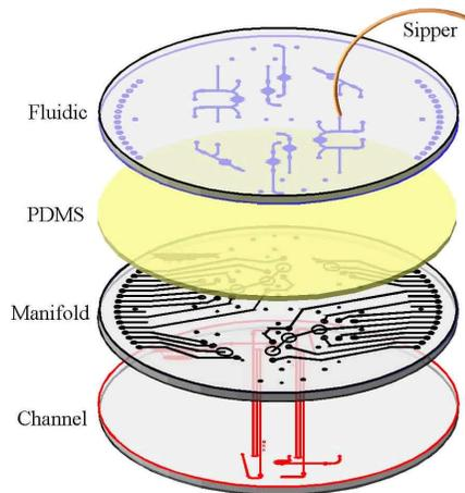
**Figure 1.** Microfabricated wafer for sample preparation and amino acid analysis. The 100-mm diameter microfabricated wafer stack is composed of a 4-layer sandwich of glass and PDMS to create channels and pumping structures.
