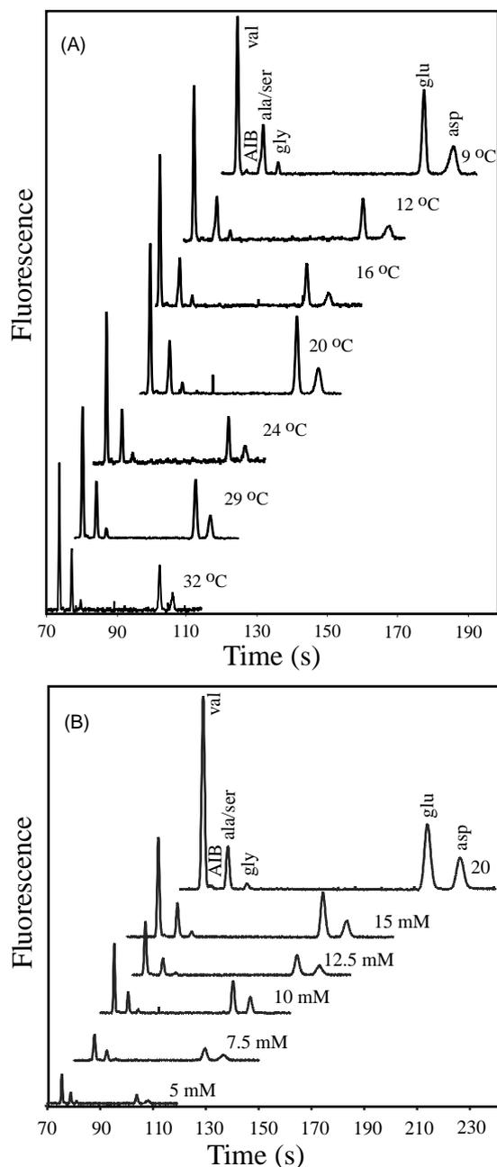
Fig. 2. (A) Temperature dependence of the capillary zone electrophoresis separation of the Mars7 Standard. Run conditions: buffer 10 mM  $\text{CO}_3^{2-}$ , pH 9.8, 700 V/cm, effective separation length 19.25 cm. (B) Ionic strength dependence of the separation of the Mars7 Standard. Run conditions: buffer pH 9.6, 700 V/cm,  $T = 8^\circ\text{C}$ , effective separation length 19.25 cm.
