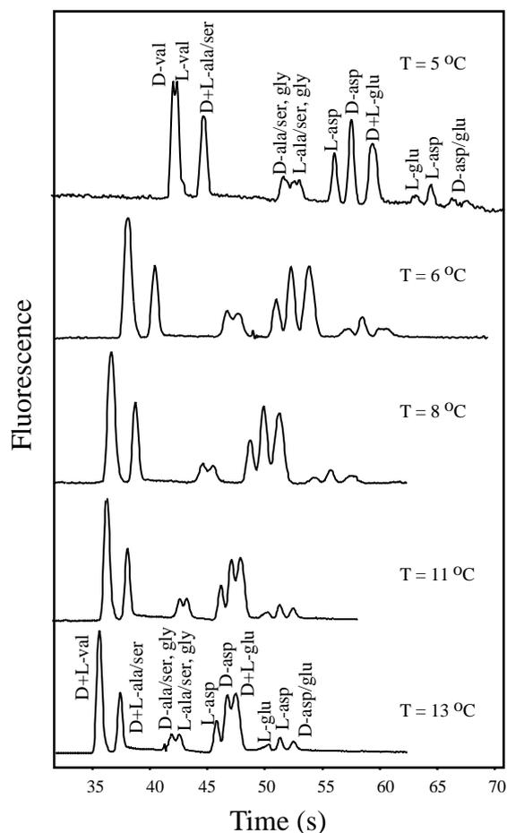
Fig. 6. Chiral separation of Mars7 Standard as a function of temperature. Run conditions: buffer 10 mM  $\text{CO}_3^{2-}$ , 15 mM HP $\beta$ CD, 700 V/cm. Effective separation length 6.2 cm. At 19.25 cm effective separation length all enantiomers are resolved at all temperatures (not shown).
