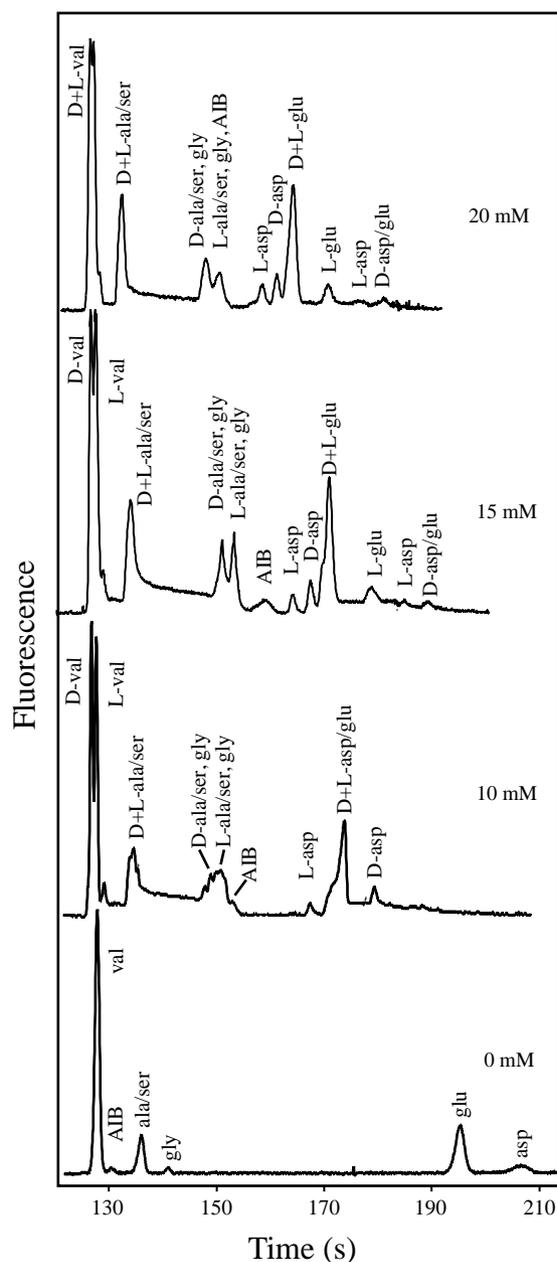
Fig. 5. Effect of HP $\beta$ CD concentration on the separation of the Mars7 Standard. Traces have been shifted slightly in time ( $<10$  s) to align the valine peaks for ease of comparison. Run conditions: buffer 10 mM  $\text{CO}_3^{2-}$ , pH 8.9, 700 V/cm,  $T = 14^\circ\text{C}$ , effective separation length 19.25 cm.
