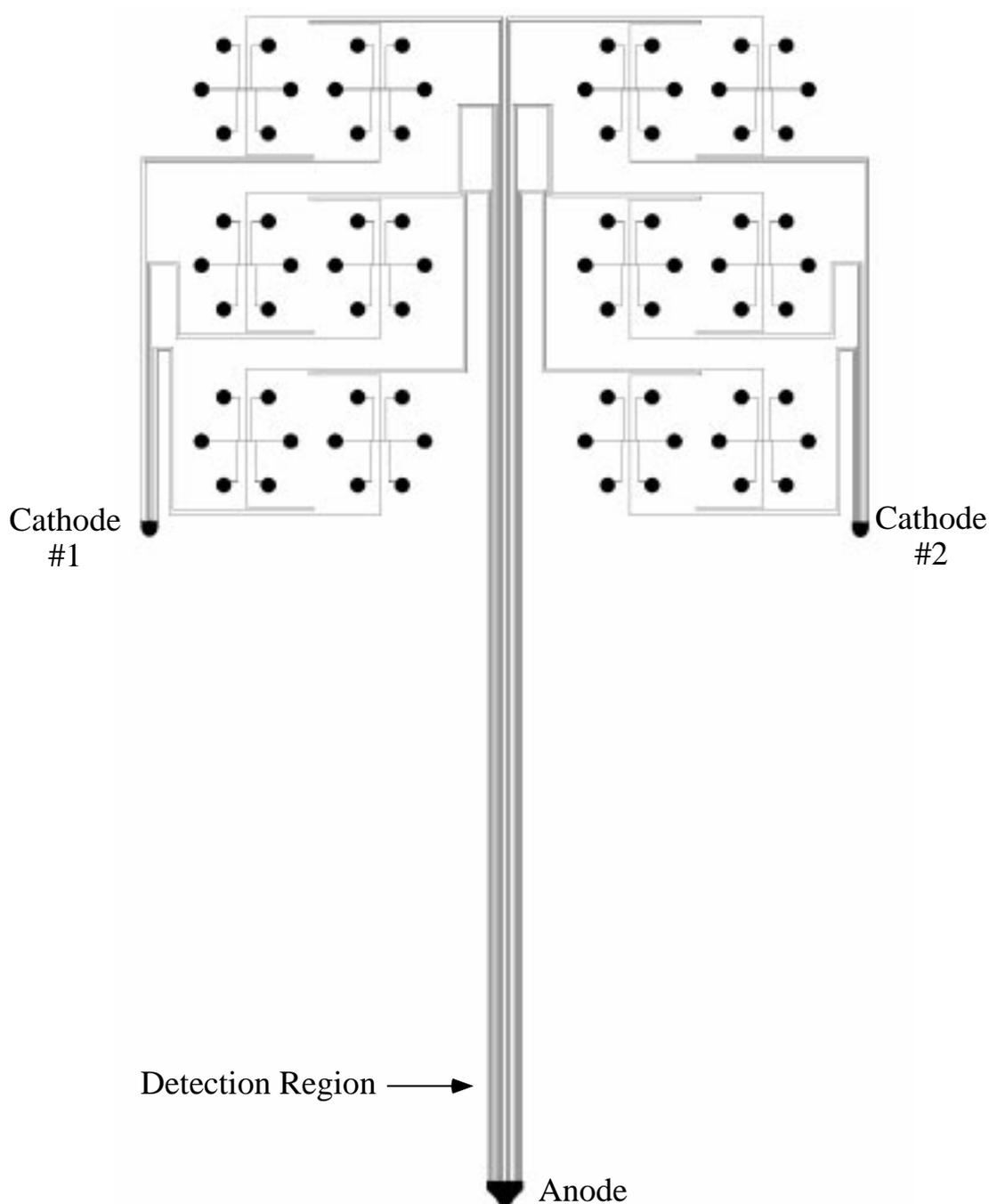
**Fig. 14.** Mask design for a 48 sample chip. The chip has 12 separation channels which allow injection of four samples per channel. Two common cathodes and one anode are used to decrease the total number of holes. The pattern fits onto a 10 cm glass wafer.
