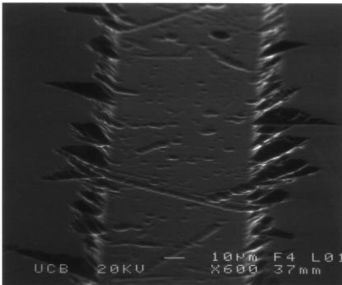
**Fig. 4.** Scanning electron micrograph of polished Borofloat etched 7  $\mu\text{m}$  using a Au/Cr etch mask. The patterns in the etched channel and defects in the side wall are due to polishing induced stresses and microscratches on the surface of the glass.
