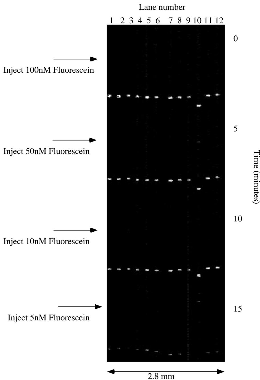
**Fig. 16.** Image of the separation of 48 samples of fluorescein on a microfabricated CAE chip. Four concentrations of fluorescein were separated in series on 12 channels. The fluorescein concentrations are 100, 50, 10 and 5 nM respectively. Total separation time is about 20 minutes.
