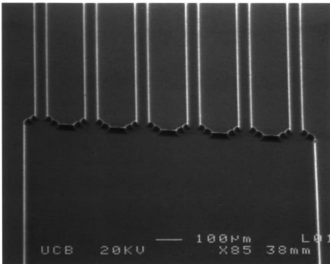
**Fig. 6.** Scanning electron micrograph showing the quality of etches in Schott Borofloat glass. The image is of the common cathode region of a 48 sample chip etched 25  $\mu\text{m}$  deep in 49% HF using amorphous silicon as an etch mask.
