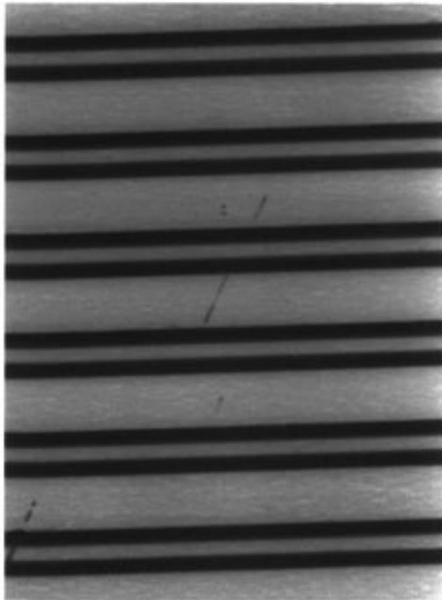
**Fig. 5.** (A) Scanning electron micrograph showing the effect of a single scratch in the glass that occurred before deposition of the protective mask. The image shows an array of channels etched 20  $\mu\text{m}$  deep in Borofloat using an amorphous silicon mask. (B) Optical image of the effect of a scratch defect in Borofloat where a pre-etch in 49% HF was performed prior to deposition of amorphous silicon and channel etching.
