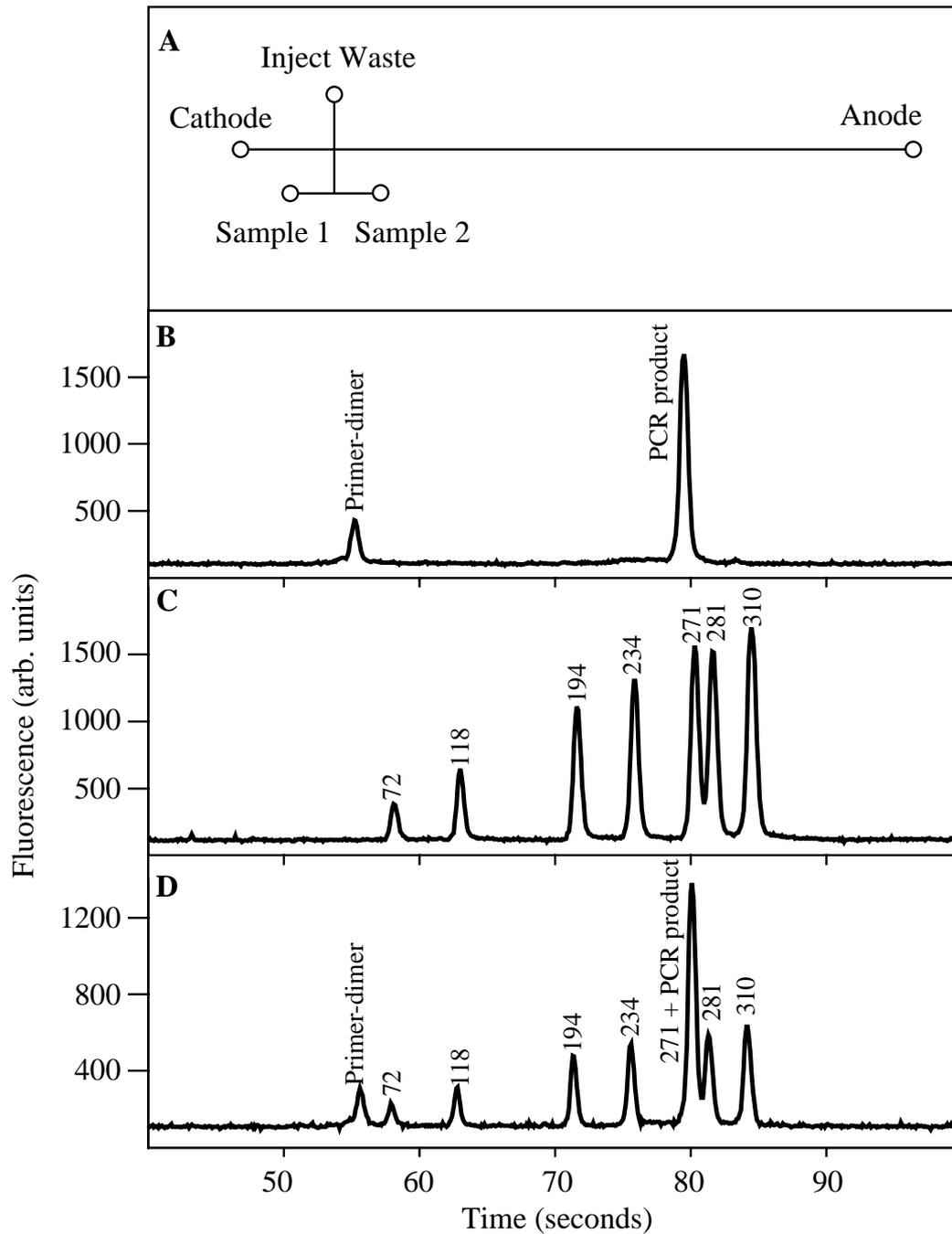
**Fig. 10.** (A) Layout of a two injection reservoir channel. Electropherograms showing serial separations of (B) a 268 bp  $\beta$ -globin PCR product, (C) the smaller peaks of  $\Phi$ X174 *Hae*III ladder and (D) the separation of both samples co-injected.
