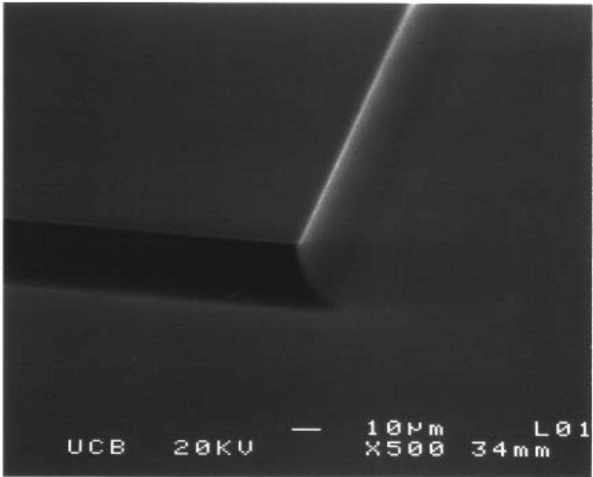
**Fig. 2.** Scanning electron micrograph showing a corner of two crossed channels etched in Borofloat. The areas to the right and bottom of the image have been etched 25  $\mu\text{m}$  deep while the area to the upper left was protected by a 1,500  $\text{\AA}$  thick amorphous silicon sacrificial etch mask.
