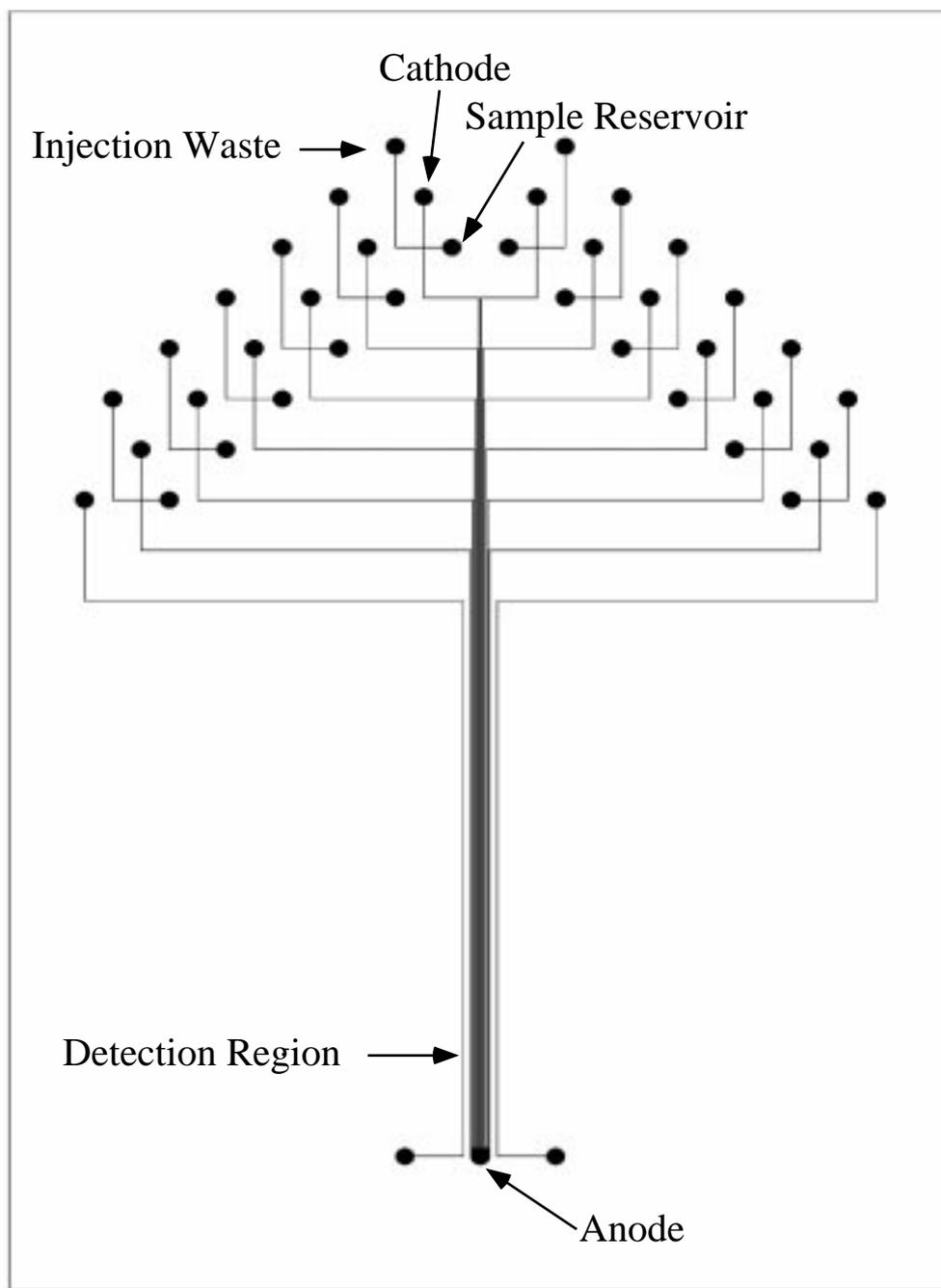
Fig. 7. Mask design used to pattern the 12 channel CAE chip. Two optical alignment channels run parallel to the separation channels. The size of the pattern (region enclosed by the box) is  $50 \times 75$  mm (Adapted from [17]).
