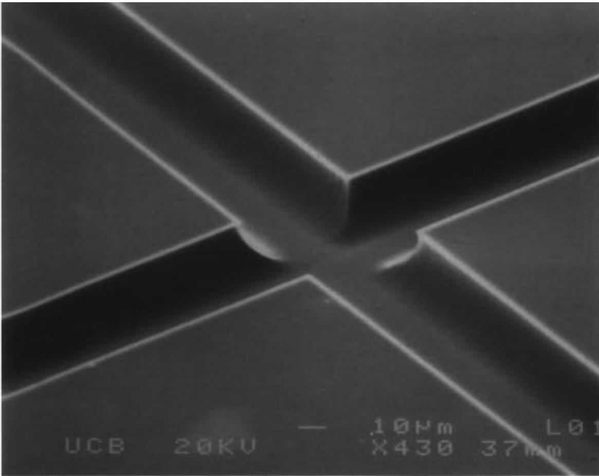
**Fig. 3.** Scanning electron micrograph of the intersection of two 25  $\mu\text{m}$  deep channels etched in Borofloat using a 1,700  $\text{\AA}$  thick amorphous silicon etch mask. Striations on the side walls of the capillary are evident near the intersection.
