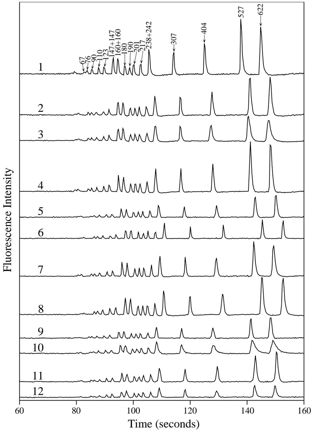
**Fig. 9.** Electropherograms of pBR322 MspI DNA (2 ng/ $\mu$ l) separations performed in parallel on the 12 channel chip. The sizes of the DNA fragments are labeled next to the respective bands detected in lane 1. The average signal for each lane as a function of time is shown; the fluorescence intensity scale is the same for all 12 electropherograms (Reproduced with permission from [17]. Copyright 1997 A.C.S.).
