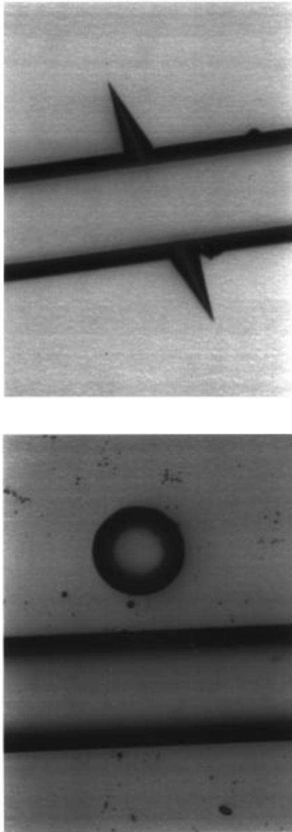
**Fig. 1.** (A) Optical image of a defect in Borofloat glass etched to a depth of  $25\ \mu\text{m}$  using 49% HF and Cr/Au ( $150\ \text{\AA}/1,500\ \text{\AA}$ ) as the etch mask. This defect is characteristic of thick Cr and Cr/Au sacrificial etch masks. (B) Optical image of a defect in a Borofloat substrate caused by a pinhole in the Cr/Au mask after an etch with 49% HF to a depth of  $25\ \mu\text{m}$ .
