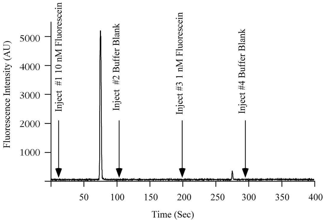
**Fig. 12.** Electropherogram studying the effects of contamination in the four sample capillary. The figure shows the separation of 10 nM fluorescein injected from reservoir 1, a buffer blank injected from reservoir 2, 1 nM fluorescein injected from reservoir 3 and again a buffer blank was injected from reservoir 4.
