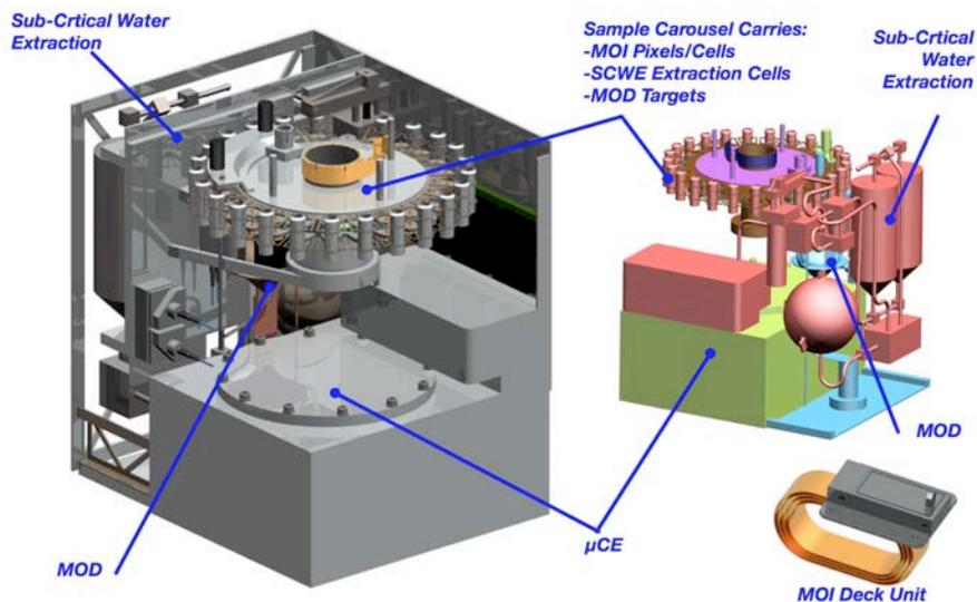
*Elements of the Urey instrument include the Mars Oxidant Instrument (MOI), the Mars Organic Detector (MOD), the MicroCapillary Electrophoresis Instrument and the Sub-critical Water Extractor (SCWE).*
